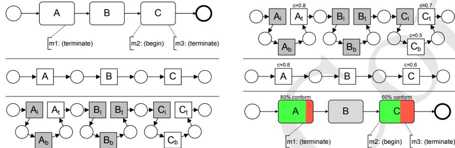
(a) Translation of an annotated operational business process in BPMN into a Petri net. The annotations describe monitoring points attached to the model at certain state transitions. First step uses translations as in [9] and the second is a postprocessing step replacing each activity with a simplistic lifecycle of *init*, *begin*, and *terminate*. The observable transitions of the resulting Petri net are white, the unobservable are marked gray.
